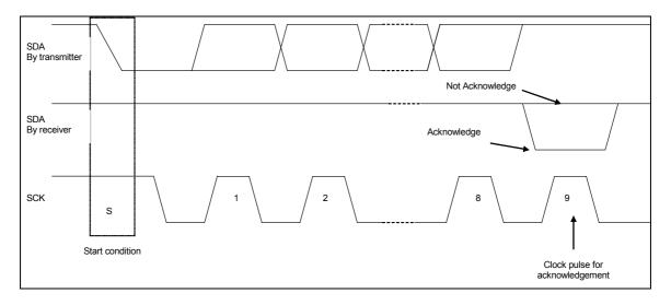
Figure 20: Waveform diagram for I<sup>2</sup>C acknowledgement on SDA
