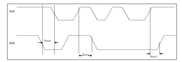
Figure 19: Waveform diagram for I<sup>2</sup>C start and stop conditions
