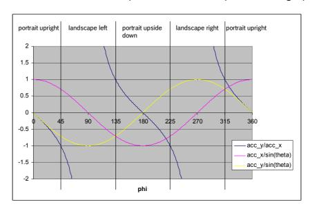
The criteria for portrait/landscape switching is fulfilled and the interrupt is generated when the threshold  $|acc_y/acc_x|=1$  is crossed (i.e. 45°, 135°, 225°, 315°). As soon as the interrupt is set, no new interrupt is generated within the hysteresis level of  $0.66 < |acc_y/acc_x| < 1.66$  corresponding to a hysteresis interval of  $\pm 13\%$  around the threshold.
