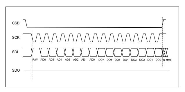
Figure 18: 3-wire SPI read protocol
