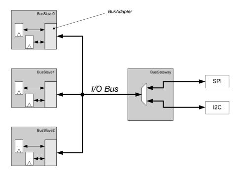
Figure 14: BMA220 I/O bus concept
