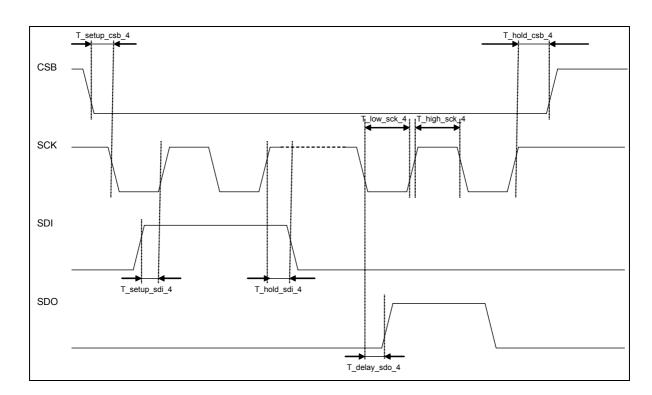
Figure 17: Timing diagram of 4-wire SPI cycle
