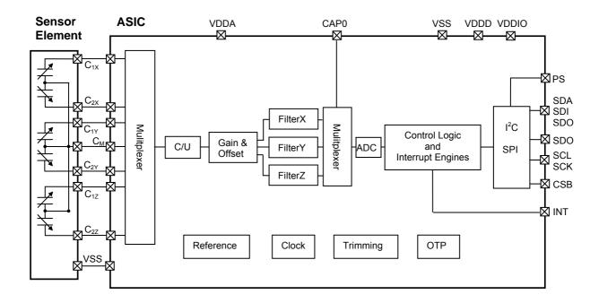
Figure 1: Block diagram BMA220
