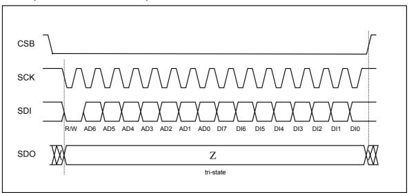
Figure 15: 4-wire SPI write command
