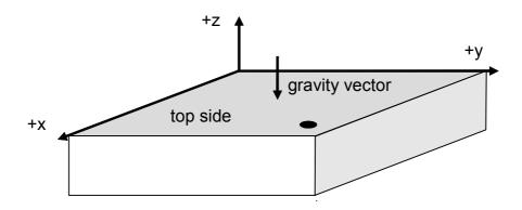
Figure 29: Orientation of sensing axes
