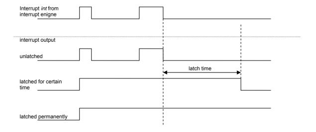
Figure 5: Interrupt output
