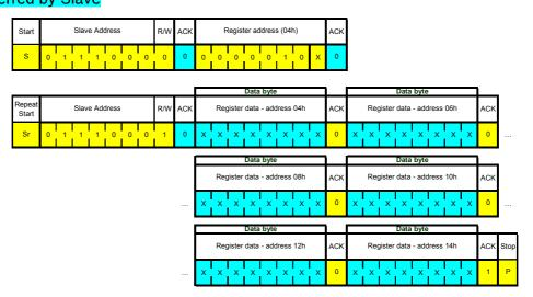
Figure 23: I<sup>2</sup>C multiple bytes read protocol
