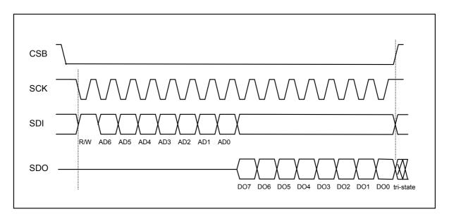
Figure 16: 4-wire SPI read command
